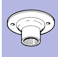
Cover, Female Dome No. R289 Material: Steel Finishes: Black Enamel, Hot Dipped Galvanised Size 20mm 25mm Standard Pack Qty 25 25
